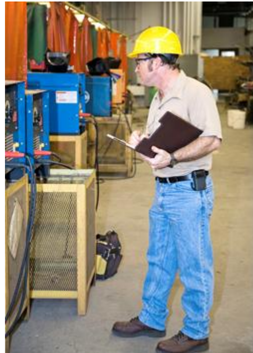
Figure 1. A maintenance audit starts with a visual evaluation of how the equipment is running, monitoring that equipment constantly throughout a work day, and recording how efficiently it is operating.
